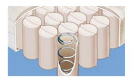
move much less than you would with other coil types. However, this also means that since each coil takes all of the weight that is put onto it by itself, and with no support from surrounding coils, the coils will provide less support for heavier people.
